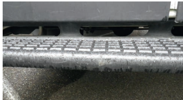
Faint scratches in the paint at the loading edges
